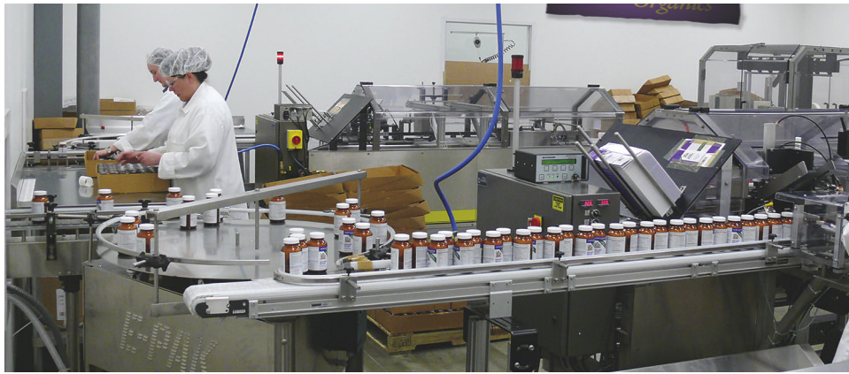
Supplement bottles convey to one of the new cartoners on the packaging line and are automatically placed in paperboard folding cartons.
