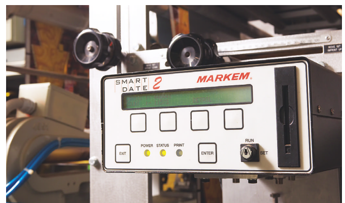
The thermal-transfer coding systems, below, are installed on a variety of vertical bagging machines like the one above. So far, Mother Parkers has 13 of the new coders at its plant in Fort Worth, used for coffee-pouch packaging.
