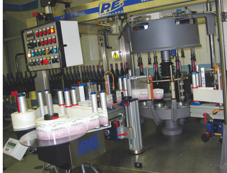
A sensor at the inlet of the labeler detects the presence of labels and triggers the label feed.
