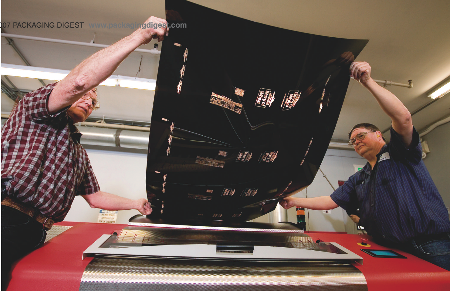
Two platemakers lift a digitally imaged flexo plate from one of flexible-packaging printer Pliant's new thermal developers.
