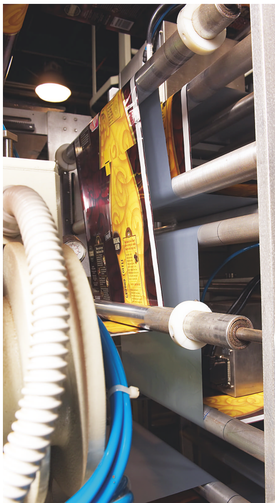
Closeup shows the coffee pouchstock unwinding through one of several vf/f/s systems Mother Parkers uses in its coffee-package production.
